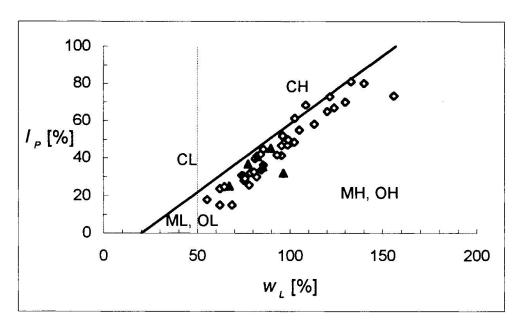
Fig. 1 Consistency characteristics of samples in plasticity chart.
