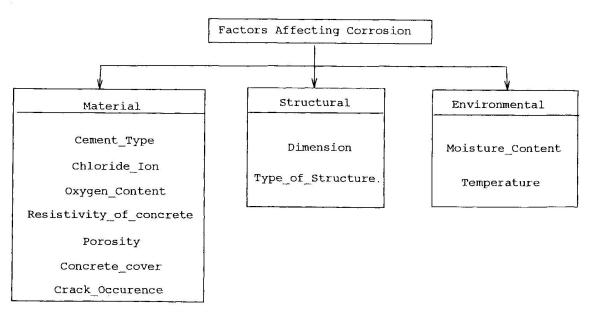
fig. 3 Factors Affecting Corrosion
