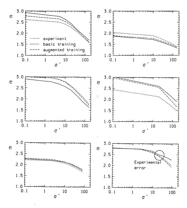
Fig. 6 Oedometer curves of the testing set.
