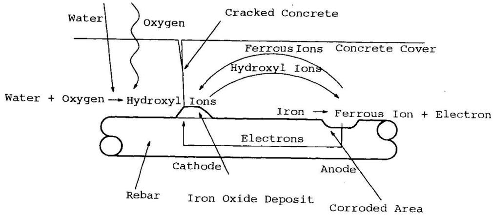
fig. 1 Corrosion Mechanism
