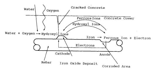
fig. 1 Corrosion Mechanism
