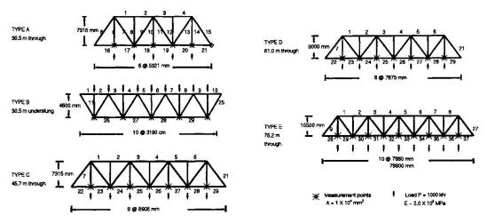
Figure 1: Configurations of steel railway bridges
