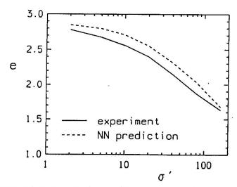
Fig. 3 Observed and preliminary determined oedometer compression lines.
