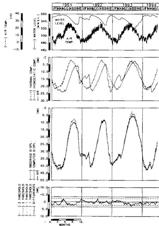
Fig.3 - Measured-Computed displacements
