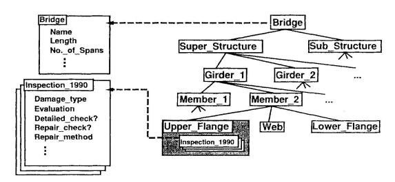
Fig.8 Example of the object-oriented representation of the bridge
