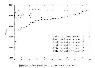
Fig.7 Repair years of the bridges
