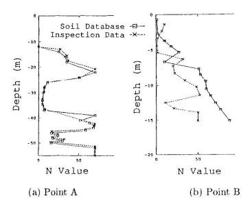
Fig.4 Comparison of standard penetration test values
