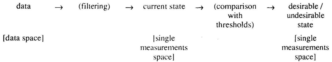
According to [5] the *domain level* contains the following concepts: *data*, *states of the type "single measurements"* (classified in current, desirable and undesirable) and *thresholds*; the *inference layer* contains *filtering* and *comparison with thresholds*; the *task level* links domain concepts and inferences generating the above written reasoning path.
