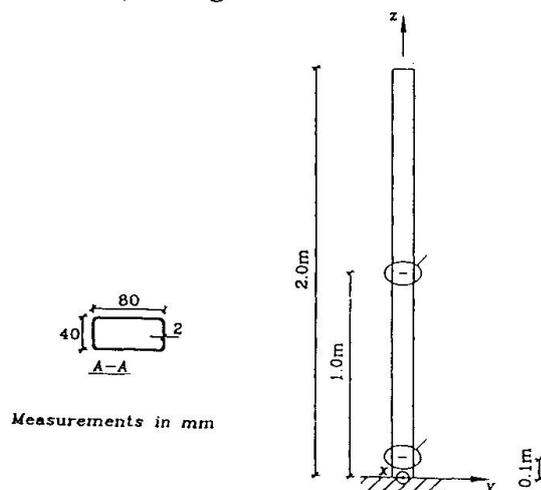
Fig. 2: Test structure.
