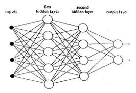
Fig. 1: Principle of a multilayer perceptron neural network.
