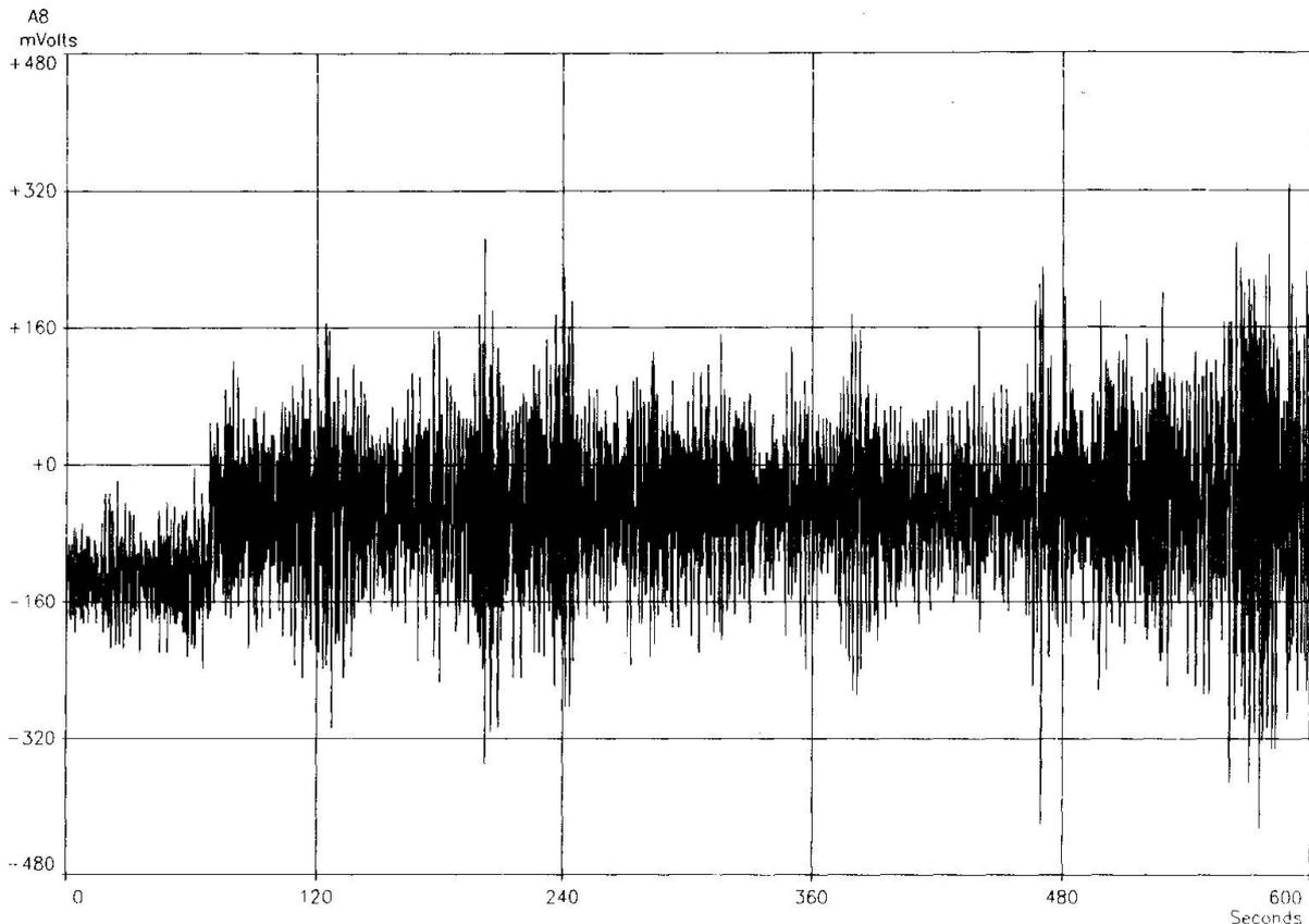
Figure 4 - Accelerometer Record Showing Change in Mean Level
