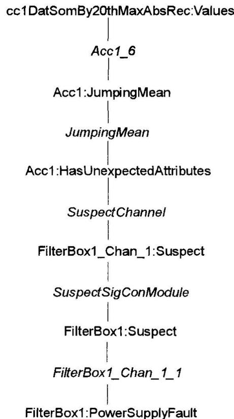
Figure 5 - Inferencing Chain For Instrumentation Fault Diagnosis
