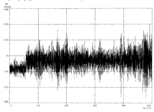
Figure 4 - Accelerometer Record Showing Change in Mean Level
