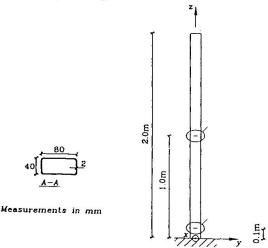
Fig. 2: Test structure.
