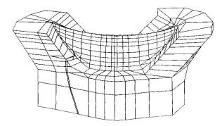
Fig.2 - 3D F.E. model of the dam
