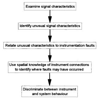
Figure 1 - Inferencing Process for Instrumentation Faults
