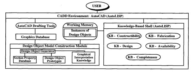
Fig. 1 SteelTeam system architecture
