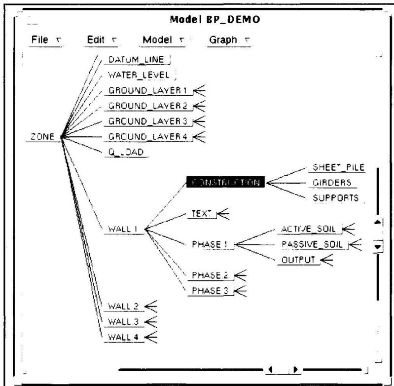
**Fig. 1** Partial product model of construction pit
