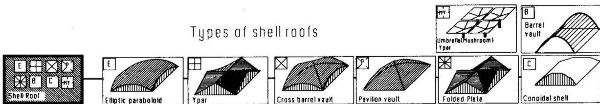
Fig.1-Reinforced/Prestressed concrete floors and roofs classification
