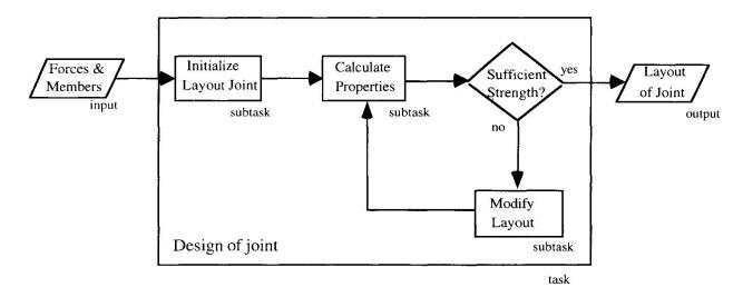
Fig. 6 Design task of a steel fabricator divided into subtasks
