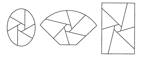
Fig.4 Reciprocal Frames over various plan shapes
