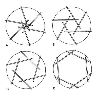
Fig.2 Plan views of retractable Reciprocal Frame structure
