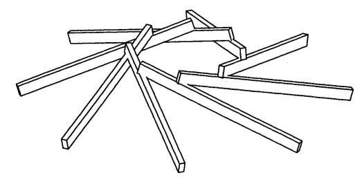
Fig.1 Three-dimensional view of Reciprocal Frame
