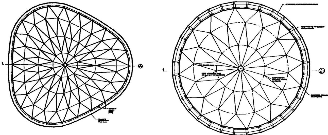
The system allows an incredible variety of alternative configurations: the plan may be a circle, a curved triangle, or an oval; the covering material may be fabric or a rigid metal deck; openings in the roof may be introduced leaving only an annular ring to cover grandstands and most exciting of all, a retractable roof can be devised.
