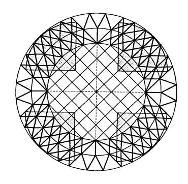
ROOF CABLE LAYOUT PLAN OPENED POSITION
