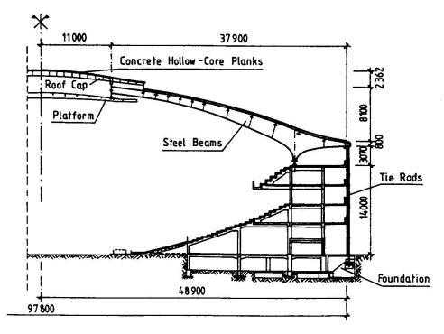
Fig. 1 Cross Section of the Westfalenhalle
