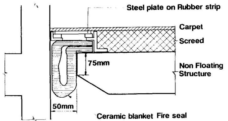
Fig.7 Railway vibration joint: isolation gaps separate all halls.
