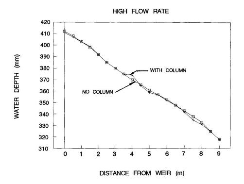
Fig.6 Sloping Gutter (1%)
