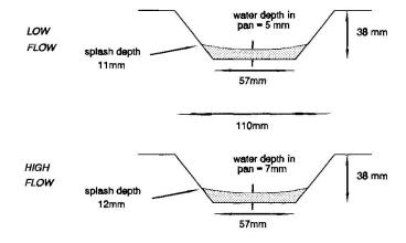
Fig.4 Depths of Flow on Roof Sheeting
