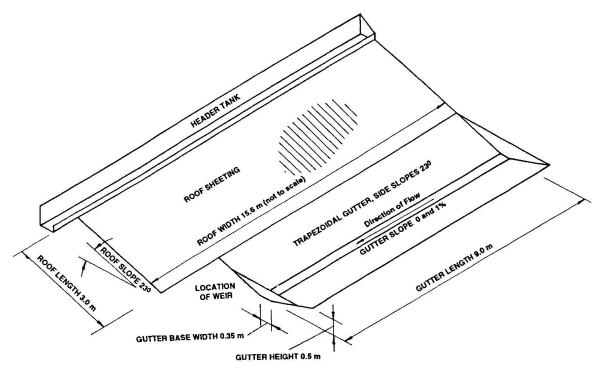
Fig.3 Model Roof and Gutter Configuration
