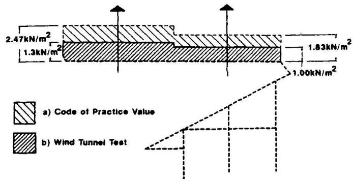
Fig 1 Murrayfield East Stand - Static Wind Pressures
