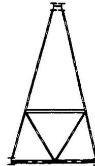
Fig 3 Leicester Main Stand Roof Girder Cross Section
