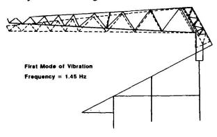
Fig 2 Murrayfield East Stand Structural Model
