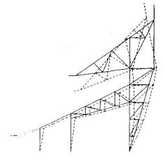
Fig. 3 First two mode shapes of a single truss
