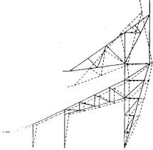
Fig. 3 First two mode shapes of a single truss
