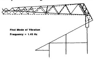
Fig 2 Murrayfield East Stand Structural Model
