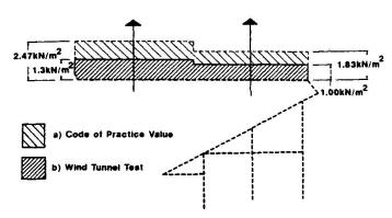
Fig 1 Murrayfield East Stand - Static Wind Pressures
