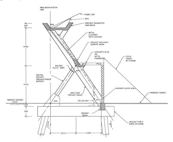
Fig. 2. Structural section
