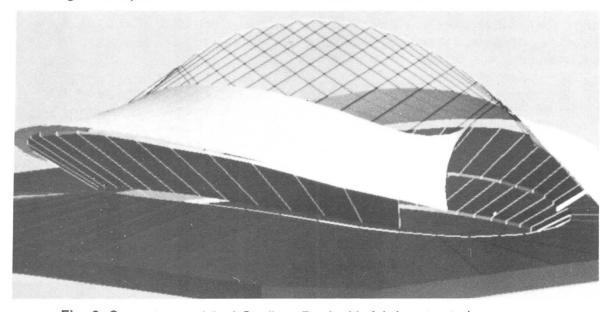
Fig. 6. Computer model of Stadium Roof with fabric retracted
