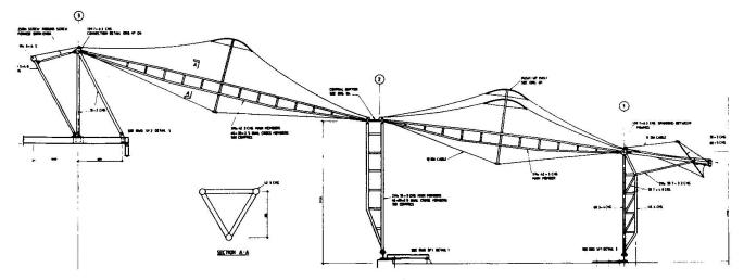
Figure 3: Section through Atrium roof
