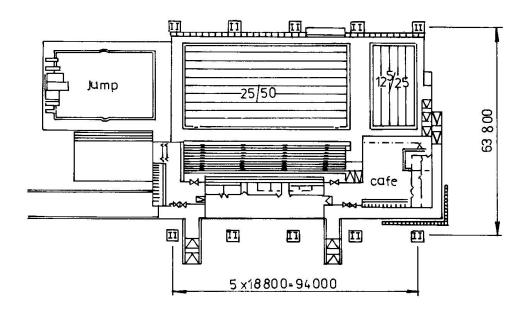
Fig. 1 Plan of the swimming complex
