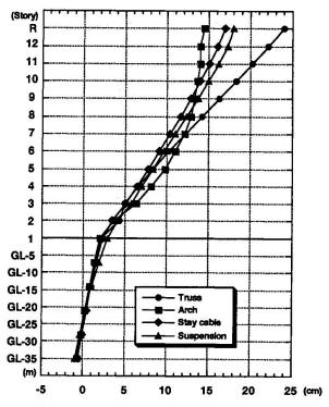
Fig. 5 Static horizontal displacements
