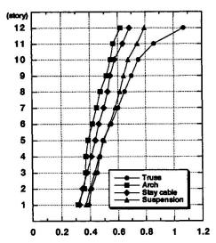
Fig. 7 Seismic story shear coefficients
