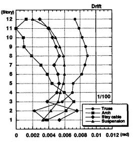
Fig. 6 Inter-story deformation angles
