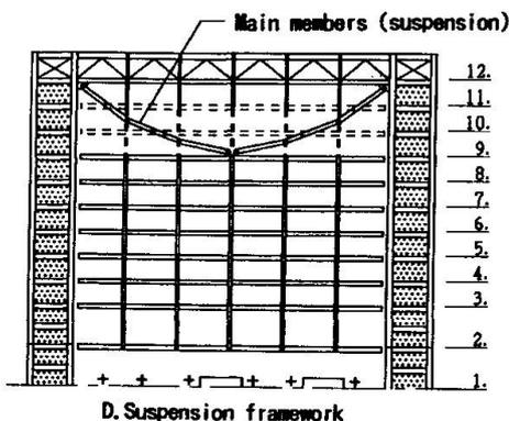
The suspended members bear only vertical loads in the part of the building above the tracks—they are not intended to bear horizontal loading. Therefore, where the suspension members intersect the beams and columns in the part of the building above the tracks, those beams and columns are paired to allow the suspension members to move freely.
