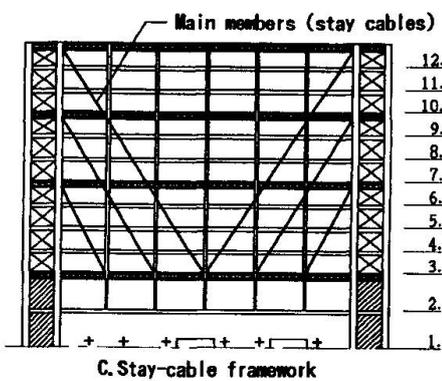
This structure is characterized in that the part of the multistory building above the tracks is suspended on cables from the core frames at either side. Beams bear the compressive forces, and the cables together with the core frames acts as effective aseismic elements.
