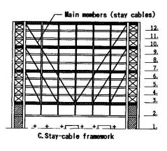
This structure is characterized in that the part of the multistory building above the tracks is suspended on cables from the core frames at either side. Beams bear the compressive forces, and the cables together with the core frames acts as effective aseismic elements.
