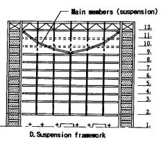
The suspended members bear only vertical loads in the part of the building above the tracks—they are not intended to bear horizontal loading. Therefore, where the suspension members intersect the beams and columns in the part of the building above the tracks, those beams and columns are paired to allow the suspension members to move freely.
