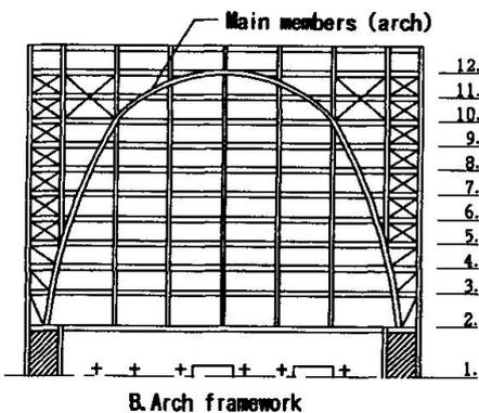
An arch is characterized in bearing both vertical and horizontal loadings. Since arches have a large cross-section and are highly rigid, bracing is provided to resist reverse shear stresses, particularly in the upper floors.
