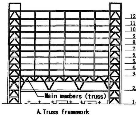
Making the first and second floors of super truss frames provides concentrated support for vertical loads. From the third floor upwards, the inner portions have a rigid-frame construction, with earthquake-resisting braces on the core frame portions on either side.
