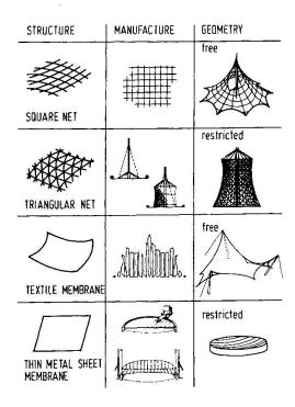
Fig. 9 Pneumatic formwork for concrete shells: suitable shapes [4]
