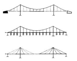
The next step towards lightness for increasing spans is to subdivide the girder into a primary structure acting either in compression (fig. 2, bottom left) or in tension (fig. 2, bottom right).
