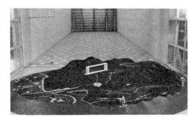
Fig.7 Wind tunnel test (monument and topographic model)
