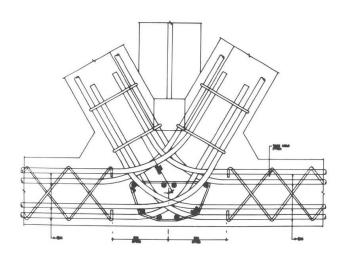
Fig 1.3 In-Situ Joint, Typical Reinforcement Detail
