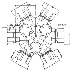
Fig. 1.2 Precast Joint Detail
