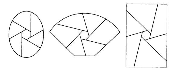
Fig.4 Reciprocal Frames over various plan shapes
