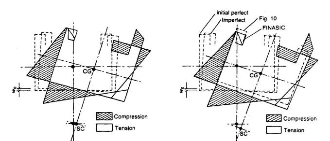
Fig.4. Comparison of Torsional buckling stresses - design model and finite element analysis
