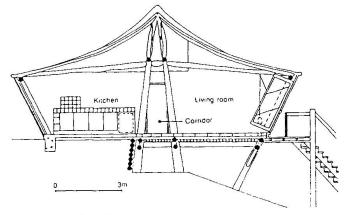
Fig. 2: Section through prototype house
