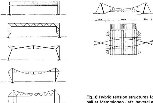
Fig. 6 Hybrid tension structures for an ice-skating hall at Memmingen (left, several alternatives) and for a multi-purpose hall at Karlsruhe [3]
