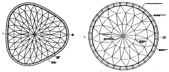
The system allows and incredible variety of alternative configurations: the plan may be a circle, a curved triangle, or an oval; the covering material may be fabric or a rigid metal deck; openings in the roof may be introduced leaving only an annular ring to cover grandstands and most exciting of all, a retractable roof can be devised.
