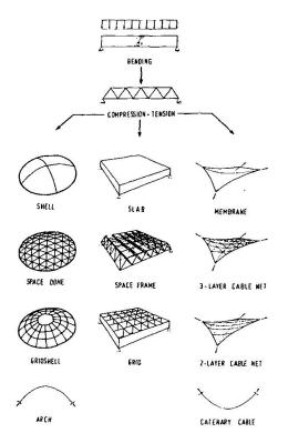
Fig. 8 The development of double-curved surface structures
