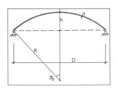
Figure 5 Measures for the structure. R = 100m, D= 123m, h = 21m and  $t_{eff} = 80mm$ .
