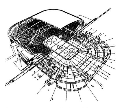
Fig. 1 Axonometric view of the Sports Hall
