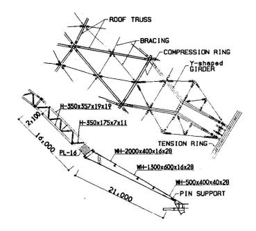
Fig. 6 Y-shaped Girder and Compression Ring
