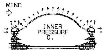
Fig.12 Max. Negative External Pressure Coefficients
