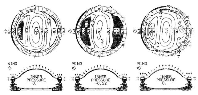
Fig.10 Average External Pressure Coefficients
