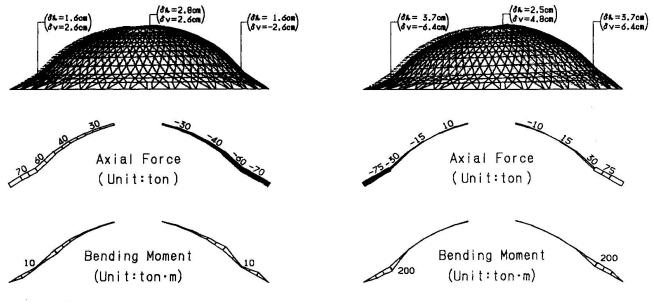
Fig. 8 Stress & Deflection due to Lateral Load
