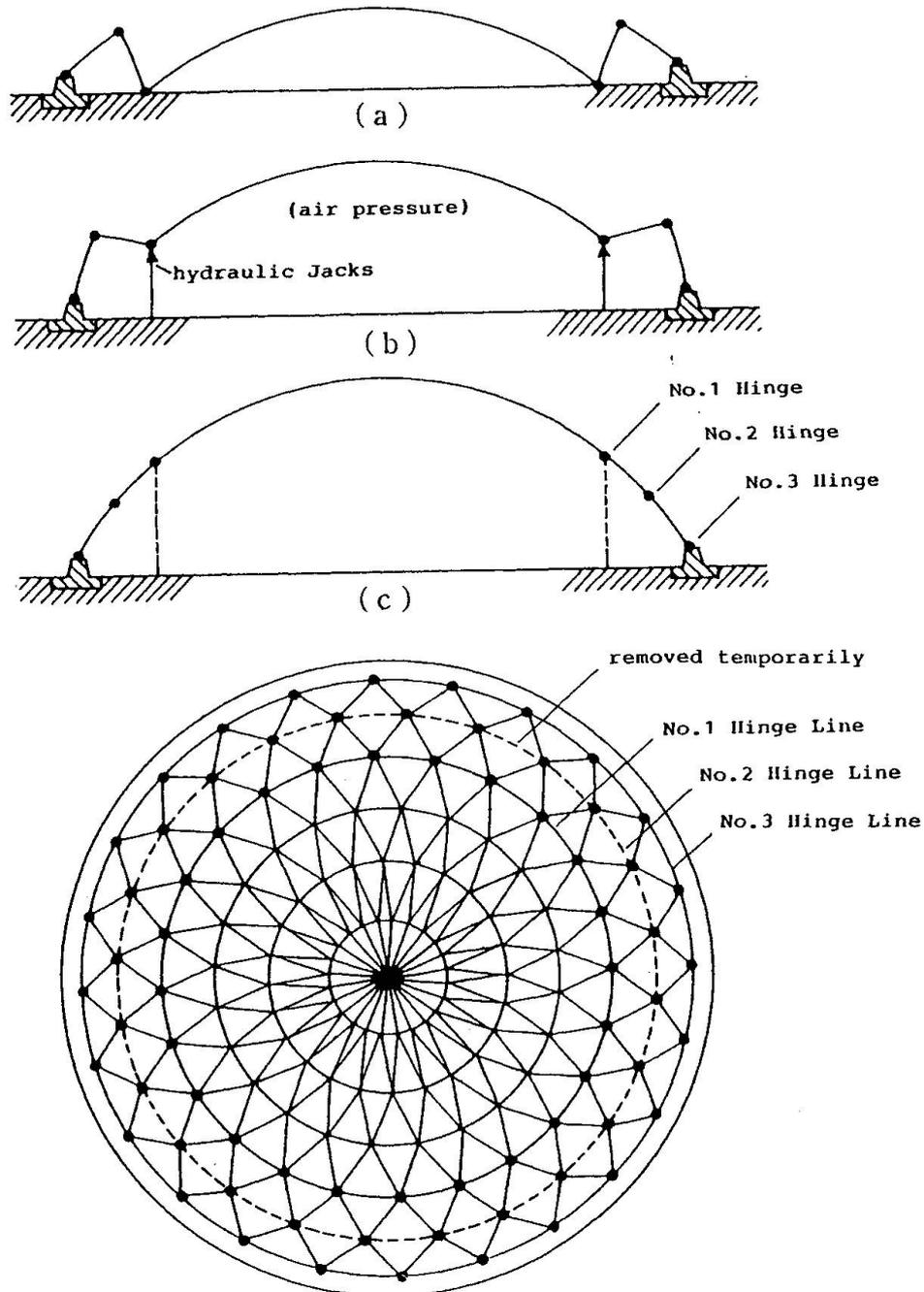
Fig. 1 Principle of Pantadome System
