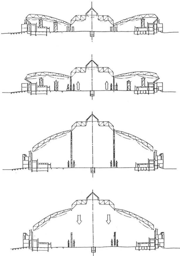
Fig. 8 Erection process
