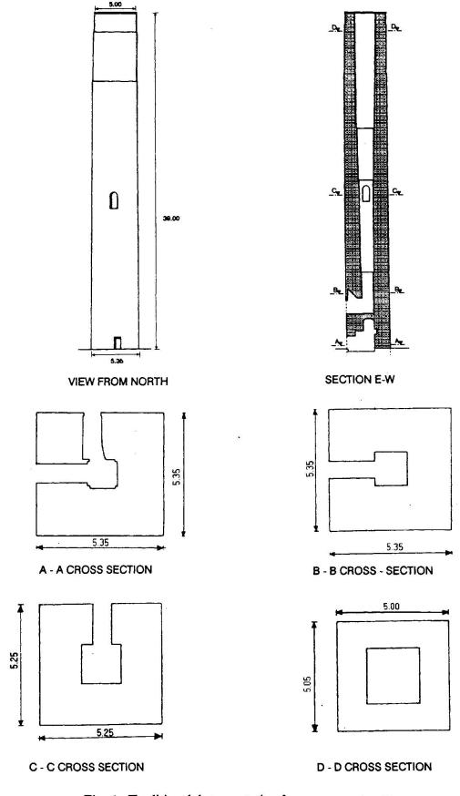
Fig. 1 - Traditional documentation for a masonry tower.
