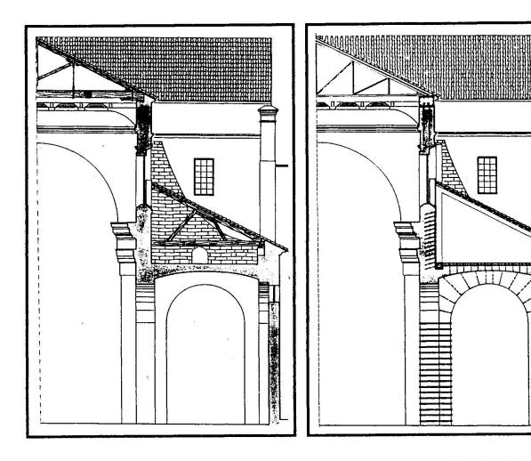
Fig. 1 Cross-section of the right side aisle before structural rehabilitation
