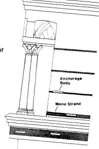
Fig. 1: Tendon Lay-Out at First Loggia
