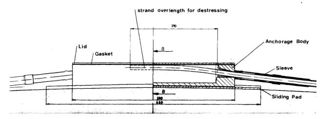
Fig. 2: Specially Designed Monostrand Anchorage Body on Sliding Pad
