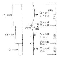
Fig 4 Bending Diagram Perpendicular to Wall
