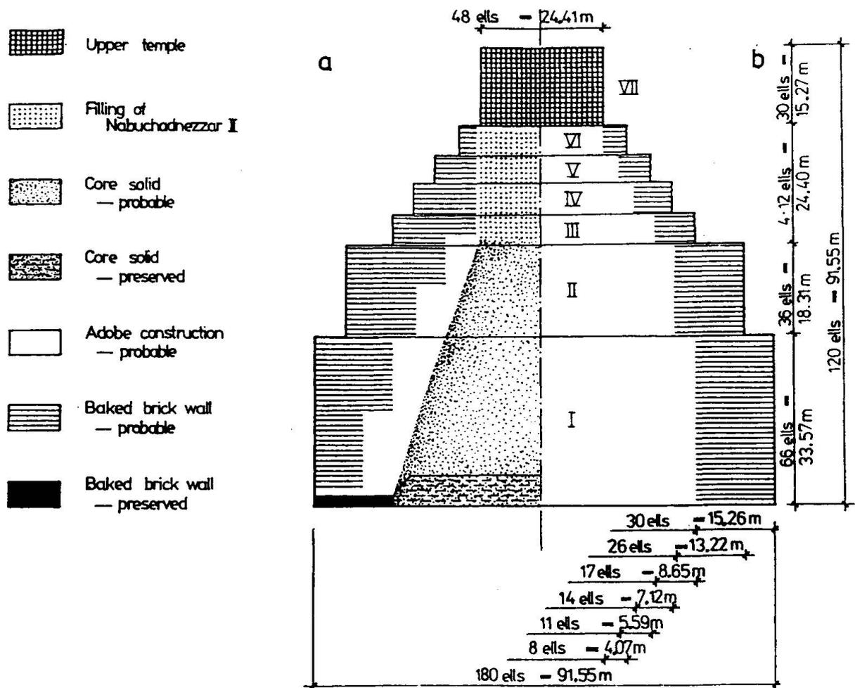
Fig. 8 Structural characteristics of the Tower of Babel - by
