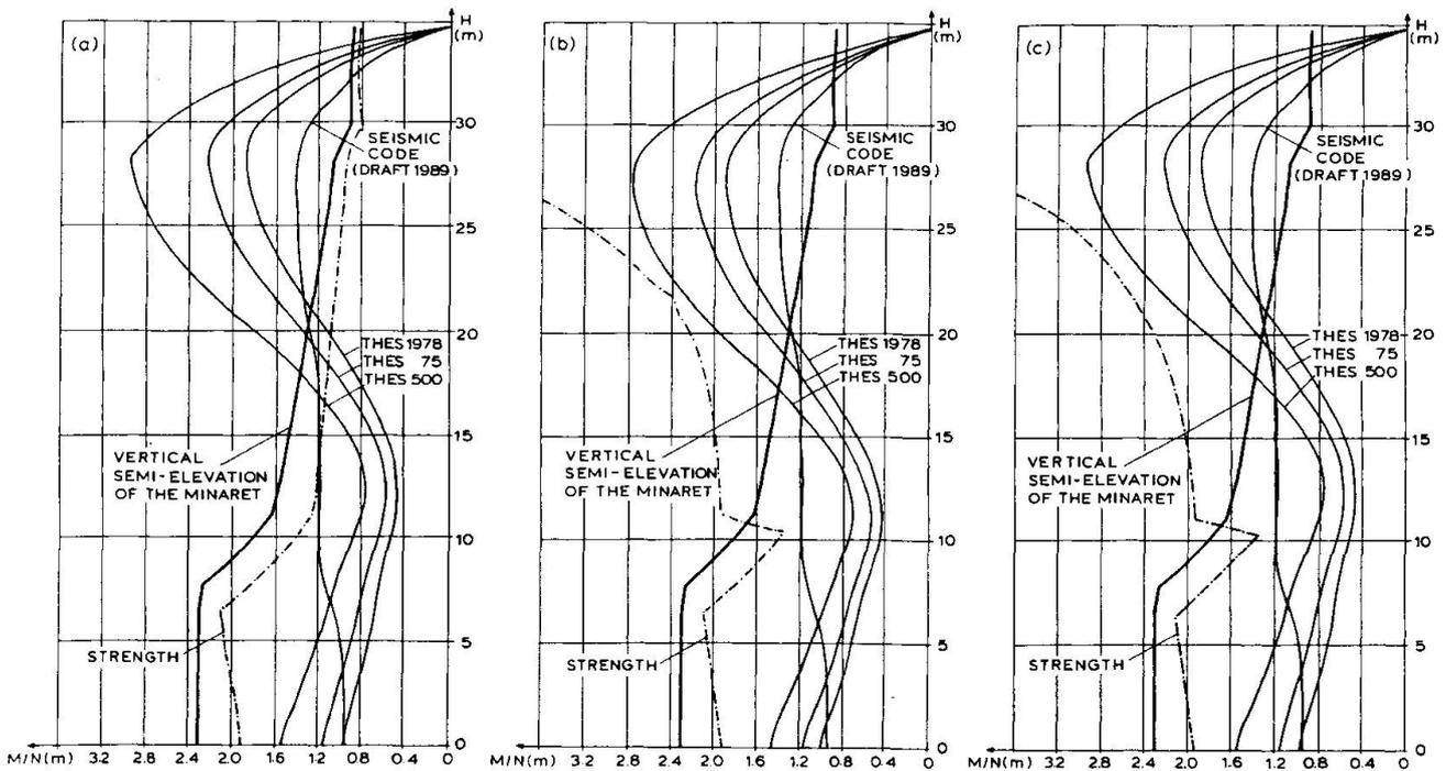
**Fig.5** Eccentricity curves under seismic spectrums and strength eccentricity curve: (a) Virginal state, (b) Concrete jacket, (c) External steel strips
