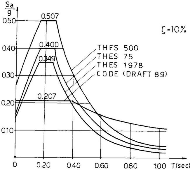
**Fig.4** Design seismic acceleration spectrums
