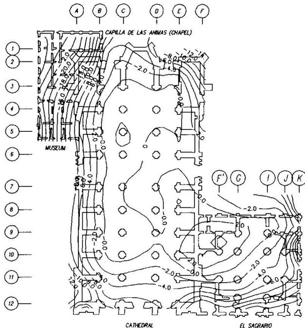
FIG 6A CONTOURS OF EQUAL SETTLEMENT RATE, IN mm/year; MEASUREMENTS FROM JAN 7, 1991 (N20) TO SEPT 2, 1991 (N28)
