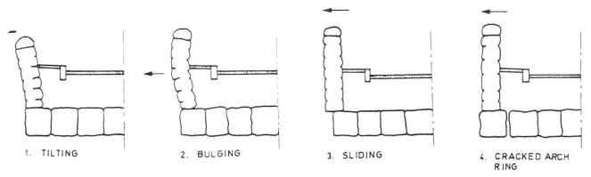
Fig 3 Spandrel wall failures
