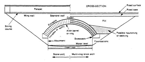
Fig 1 Typical masonry arch bridge construction
