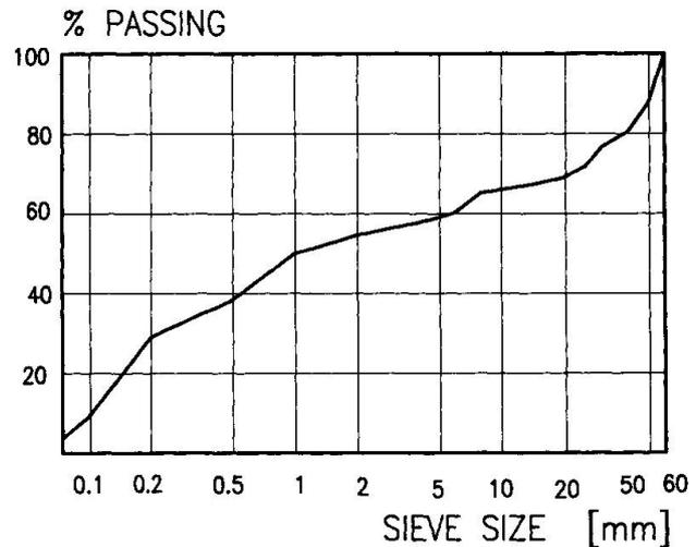
Fig. 2 Grain size of the fill material
