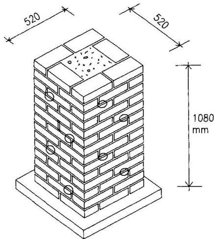
Fig. 1 Test column showing arrangement of connectors
