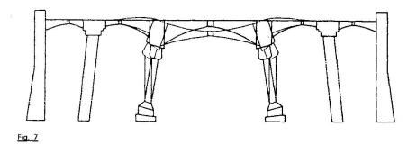
Except in the zone close to the moving capitals, the distribution of forces obtained at the level of the arches and ribs remains similar to that of a funicular type of equilibrium, although the geometry does not correspond to that of the model. It
