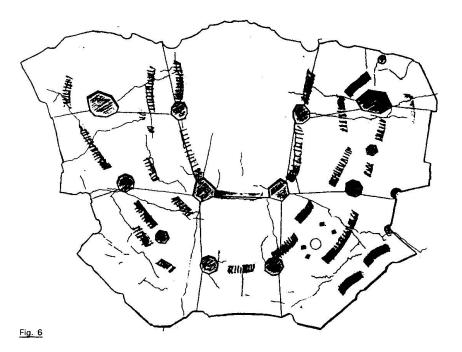
The figure 6 is a plan of the solera which shows the gaps provided to leave room for the columns of the church above, which no doubt is relevant to the matter of shrinkage. On this plan, if we observe the numerical forecasts and the present evaluations which recommend the provision of walls with expansion joints every eight metres, and if we look for the areas where, because of their smaller cross-section and a geometry which might provoke cracking, assuming uniform grid, we reach
