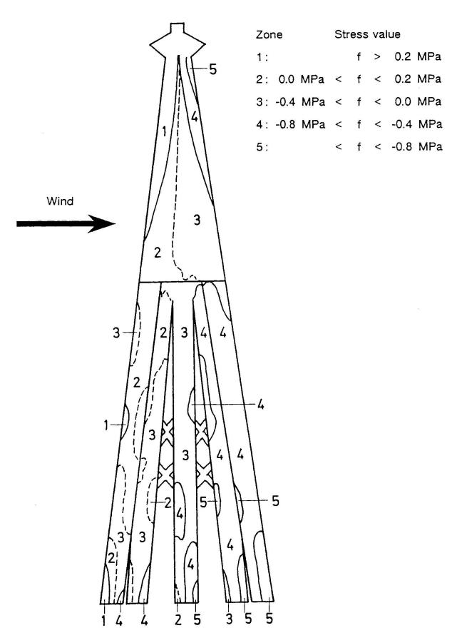
Fig. 3 Vertical stress distribution in the spire under self weight and wind loading
