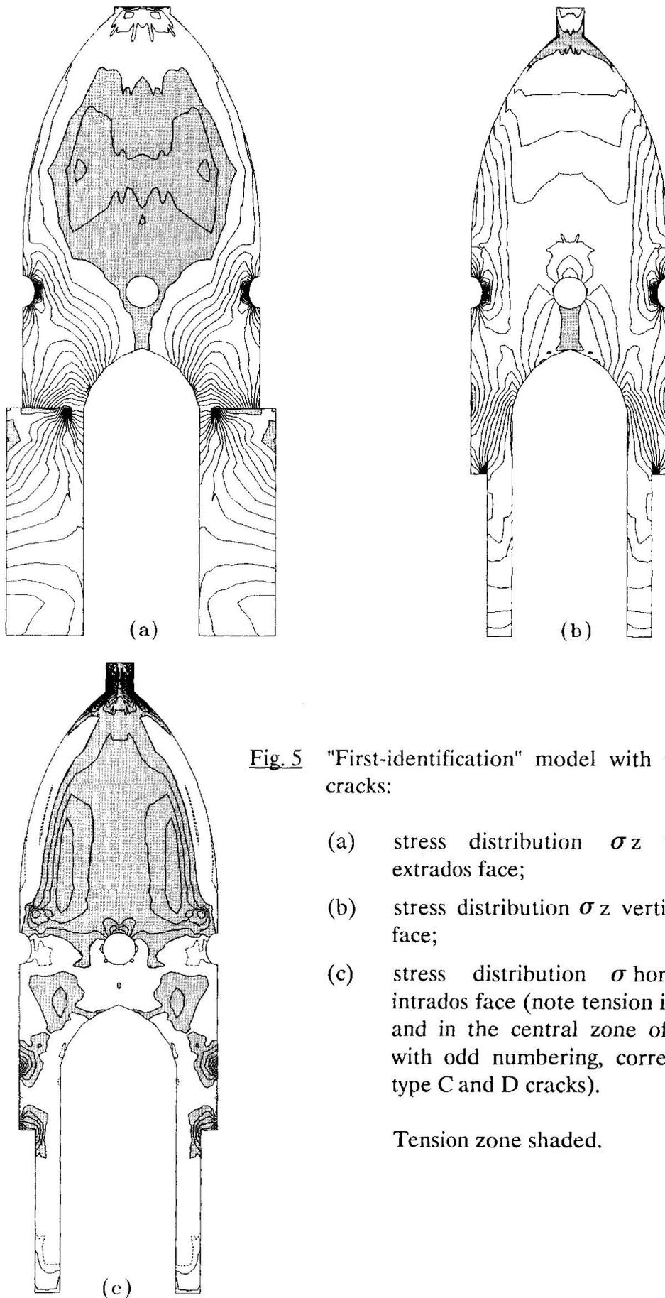
**Fig. 5** "First-identification" model with type A and B cracks:
