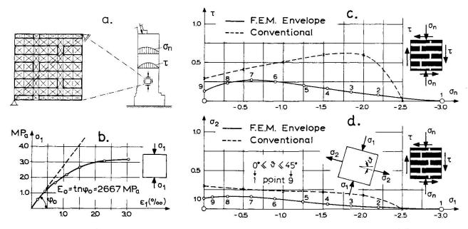
Fig.2 Analytical evaluation of masonry properties: a.Masonry micromodel, b.Stress-strain curve  $(\sigma_n - \epsilon_n)$ , c.Failure envelope  $(\sigma_n, \tau)$ , d.Failure envelope  $(\sigma_1, \sigma_2)$
