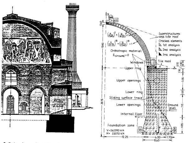
Fig.5 Rotunda: a.Meridional cross section, b.Axisymmetric F.E. model, predicted cracking
