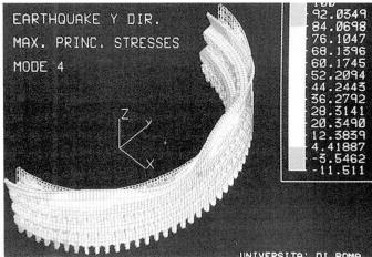
fig. 3 - 4 Response spectrum dynamic analysis for the original shape
