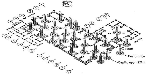
$\underline{\text{Fig. 10}}$  Position of the main shafts and radial perforations for the correction of the differential settlements
