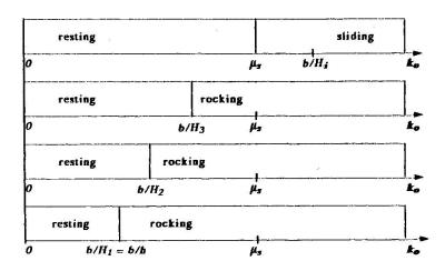
FIG. 8. Starting modes for multiblock column.
