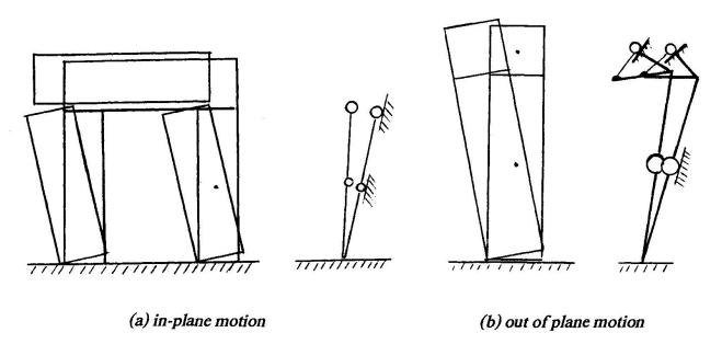
FIG. 9. One d.o.f. trilith mechanism.
