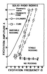
Fig. 7. Summary of sinusoidal tests for solids
