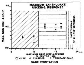
Fig. 9. Maximum earthquake rocking response
