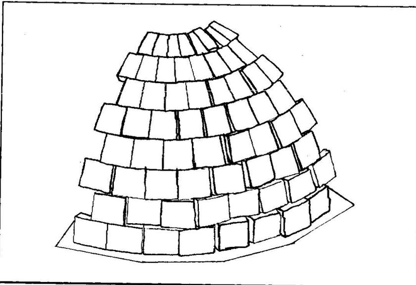
fig.2-A 90° sector of a spherical dome subjected to horizontal outward action on the second row
