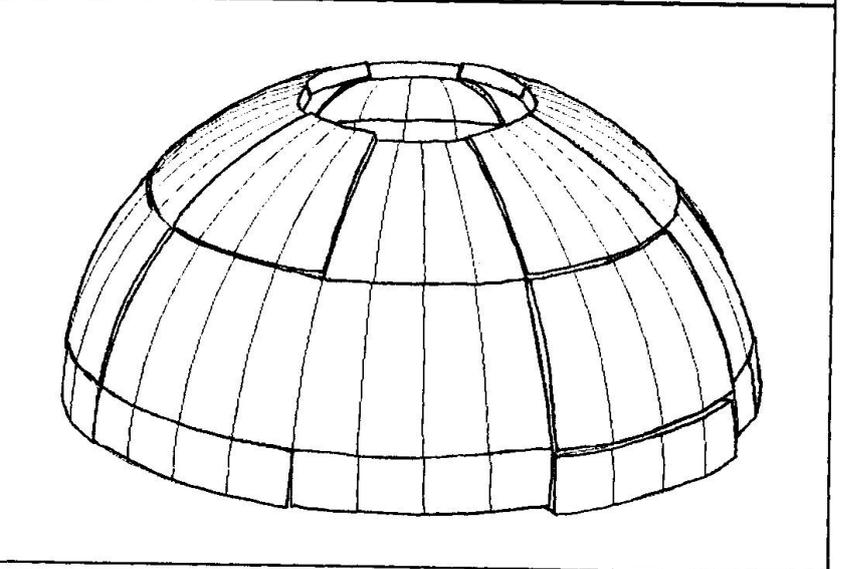
fig.4 - Global collapse mechanism for a spherical dome with hinges positioned at 45° and 80° for the settlement of one basis.
