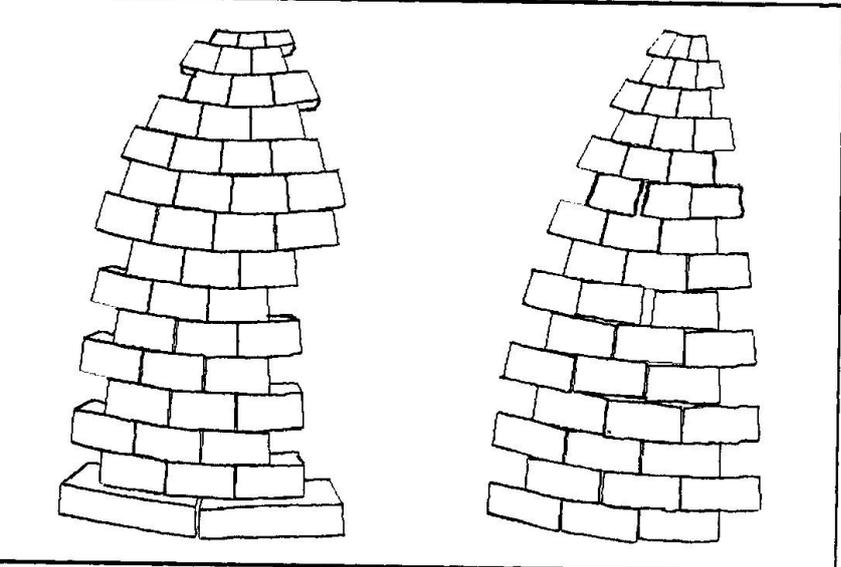
fig. 3 - Collapse mechanism for a 45° sector of the experimental dome ( $\lambda = 0.55$ ) and of a spherical dome ( $\lambda = 0.325$ ) for outward horizontal sliding of the base
