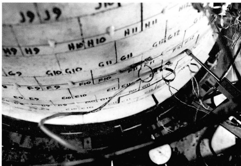
fig. 7 - Crack pattern for outward horizontal sliding of the base
