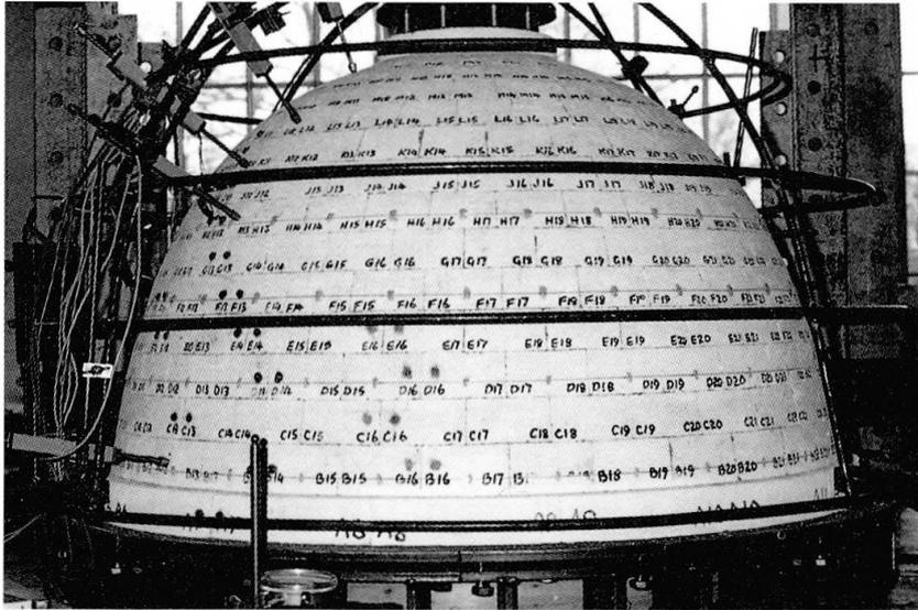
fig.6- The model dome is realised with 380 small concret blocks casted in situ. To simulate the friction characteristics of the stone sand-paper has been interposed between surfaces.
