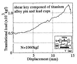
Fig.14 Load-displacement relationship of the monotonic loading tests of the drums with shear key composed of titanium pin and lead cups
