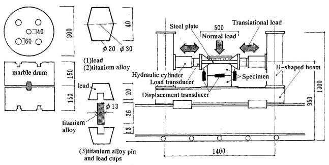
Fig.11 Model marble drums and shear keys for the static shear tests
