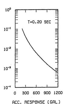
Fig.1 Seismic hazard curve for the control natural period of 0.2sec
