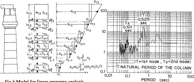
Fig.6 Model for linear response analysis of a masonry column with a beam and a pediment on its capital (Model(A))
