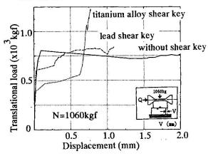
Fig.13 Load-displacement relationship of the monotonic loading tests of the drums with lead shear key, with titanium shear key, and without shear key
