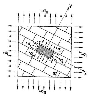
Fig. 2 Test set-up, assumption of a homogeneous state of stress
