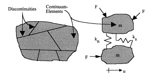
Fig. 4 Basic separation in a Distinct Element formulation
