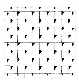
Fig. 6 Modeled brick rotations in shear stressed masonry
